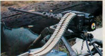
LEFT: Toxic fume levels less than five percent of self-powered MGs make EX-34 Hughes Chain Gun a top competitor in turret or cupola installations.
